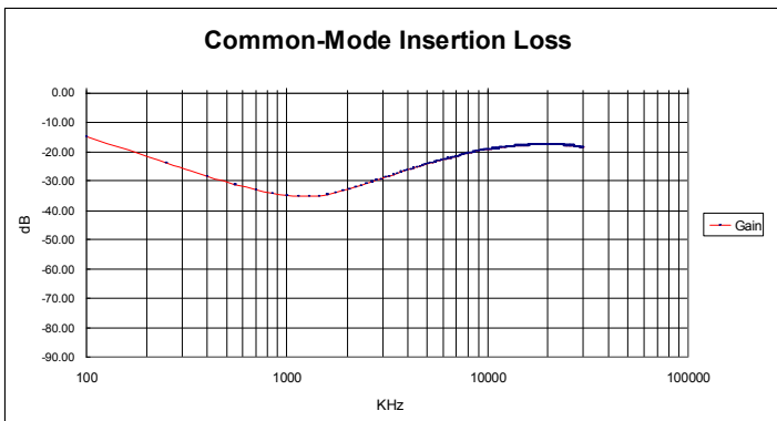
Figure 2. Typical Common-Mode Insertion Loss
