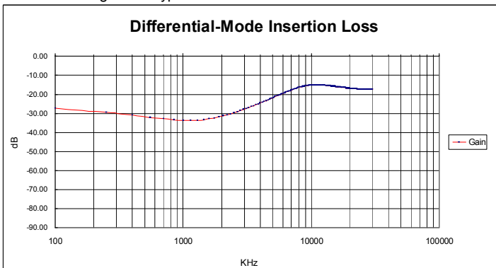
Figure 3. Typical Differential-Mode Insertion Loss
