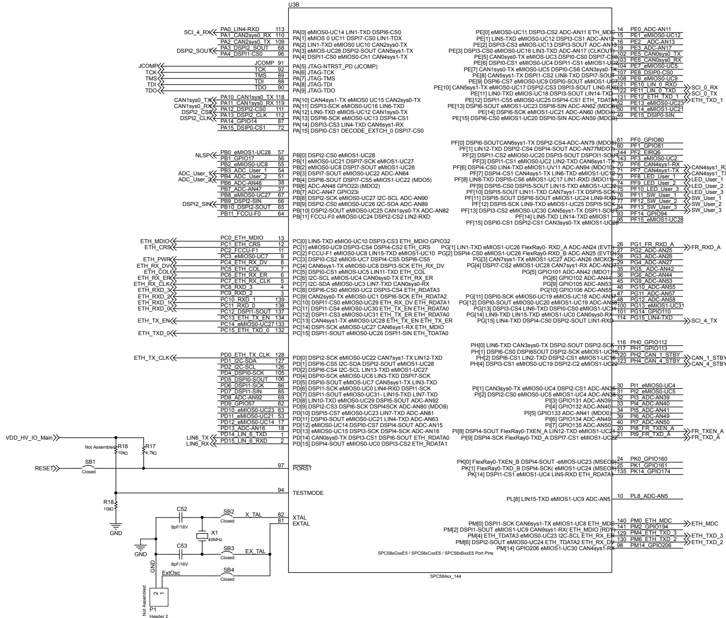
Figure 12. AEK-MCU-C4MLIT1 schematic - MCU I/O signals
